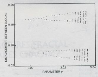
Period doubling in the behavior of two elastically coupled blocks with equal masses but subject to different friction forces.9 The graph plots the displacement between the two blocks at the end of a slip as a function of a system parameter  $\gamma$ . As  $\gamma$  increases, the system tends toward two phase-space points, then four and so forth.
